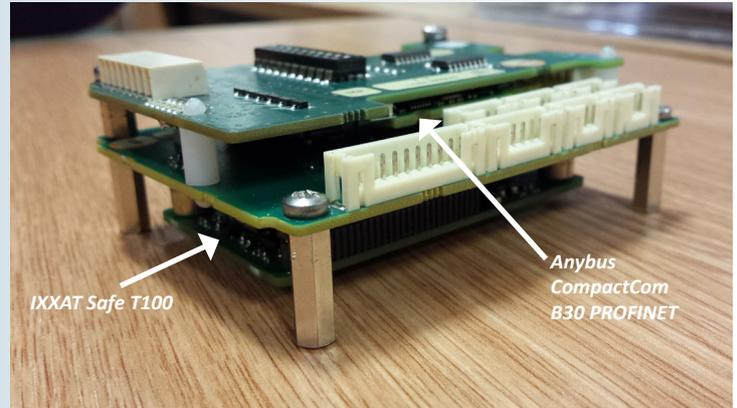
**What safety looks like.** The IXXAT Safe T100 implements the PROFIsafe layer and the safe control of three dual-channel inputs, as well as one dual-channel output. The Anybus CompactCom handles the unsafe communication and routes the safety communication to the IXXAT T100 via the black channel.
